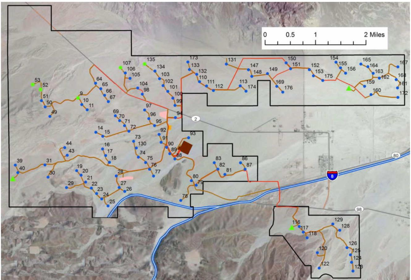
Figure 1: Turbine Layout at the Ocotillo Project
